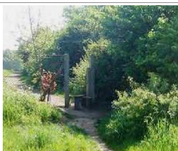
This stile is very inconvenient and denies access to a wide range of path users. Better to replace it with a single bollard or a ‘cattle grid’ if necessary. (Queens Park, Bedford)
