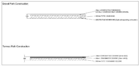
Figure 8 – Example of detail from guidelines (path surface)
