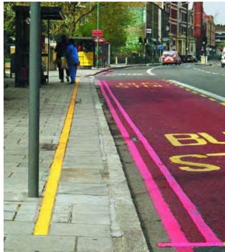
Also shown in Figure 3.13 is a yellow footway guidance line, offset 450mm from the kerb edge and 100mm in width. Guidance lines can aid drivers on their approach to stops by providing a reference point, and can also encourage pedestrians to stand away from the kerb edge. They are particularly useful at stops where limited stop services are passing without stopping.
