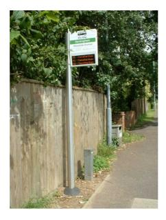
Figure 8.19: Solar-powered Real Time Information Flag
