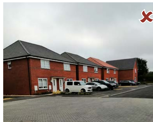
Extensive areas of hardstanding should be avoided, particularly at the front of homes.
