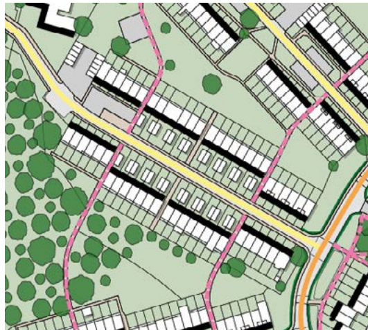
Experimental suburb with unclear distinction between the fronts and backs of buildings here showing garages sticking out on the frontage.
