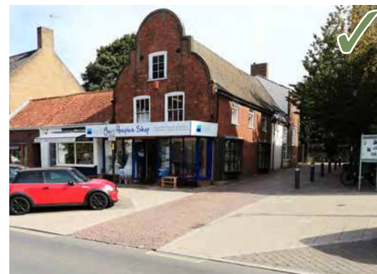
Materials and street surfaces can be used to mark different uses, users and street types, here demarcating parking spaces, pedestrian-only routes and shared surfaces in Swaffham. Non-standard materials need to be discussed with the highways authority, Norfolk County Council.
