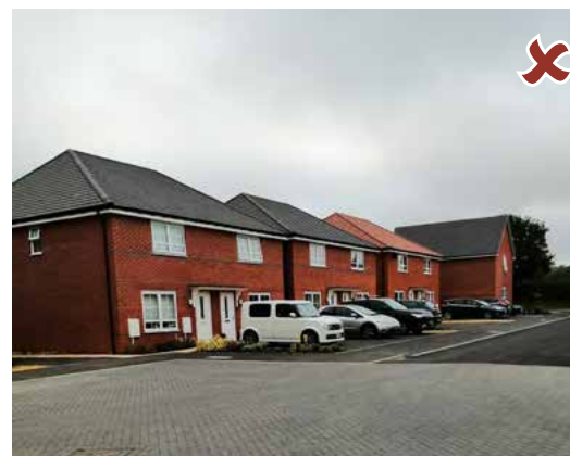
Extensive areas of hardstanding should be avoided, particularly at the front of homes.
