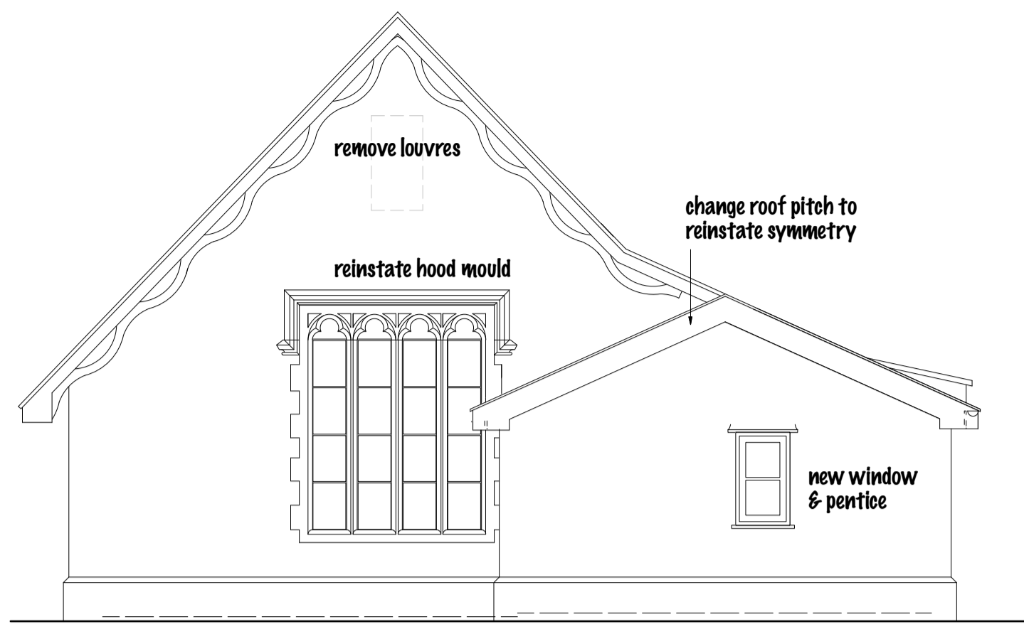
existing cement render removed clay lump repaired as required & coated with lime plaster & limewashed brick plinth repaired as required new window & pentice south elevation
