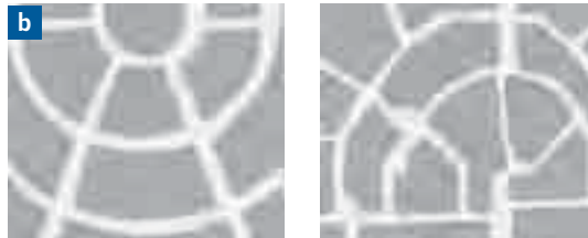
b Concentric grids designed to promote access to local centres or public transport routes.
