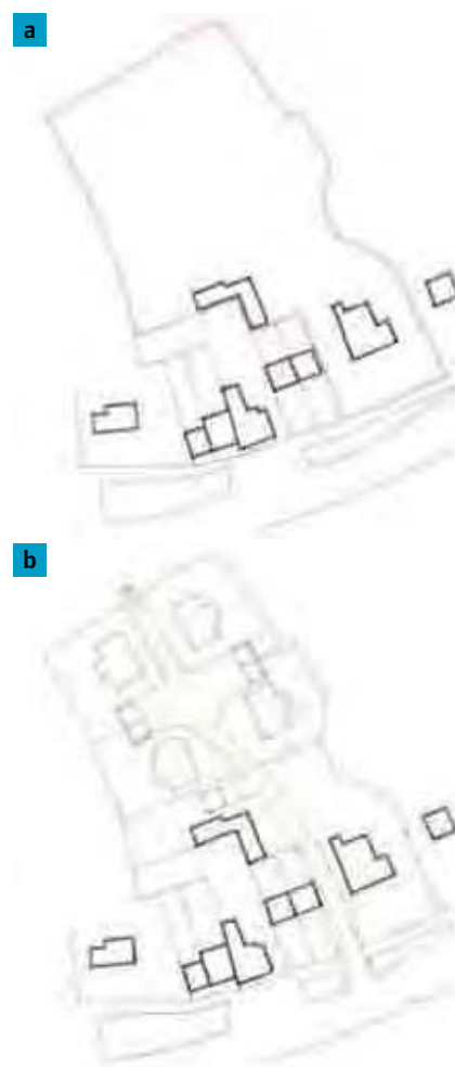
Figure 3.7 Small scheme design for an infill development (a) outlined in red. Location of new houses (b) shown in green together with new access street. Note that the new access street can be extended to allow for future growth at the top of the diagram.
