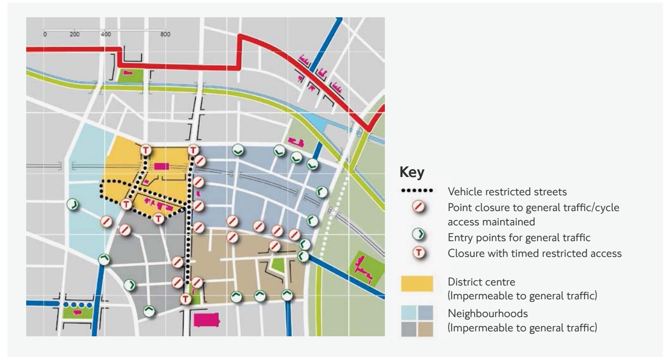
Figure 2.13 Filtered permeability area treatment example
